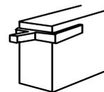
**Type 8 - Horizontal metal peg fixed to top of headstock**
